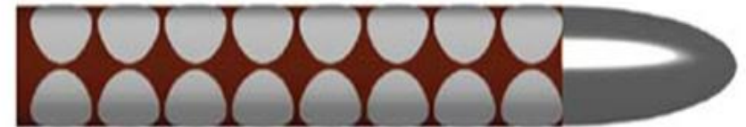
Current DBS Electrode 3 mm Cylinder Concept Design for Next Gen DBS (NeuroNexus)
